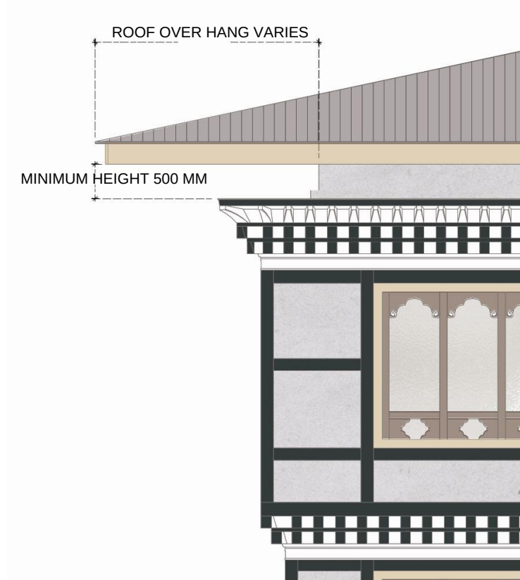
The space between eaves board and Phakhep
